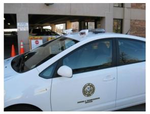
Mobile License Plate Recognition (LPR) systems are comprised of a vehicle mounted camera system and on-board computer that scans and records license plate numbers and matches unique license plate numbers against allowed plate numbers. In this way, LPR can be used to manage permit parking where a hang-tag, sticker or decal is currently used. Permitless parking is seen by many as superior to
