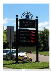
is then relayed from the meter to any mobile device (with the appropriate app) or computer. Parking facilities use the revenue and access control systems to determine space availability and then provide this information externally or signs can be mounted on the exterior of the facility to indicate space availability.
